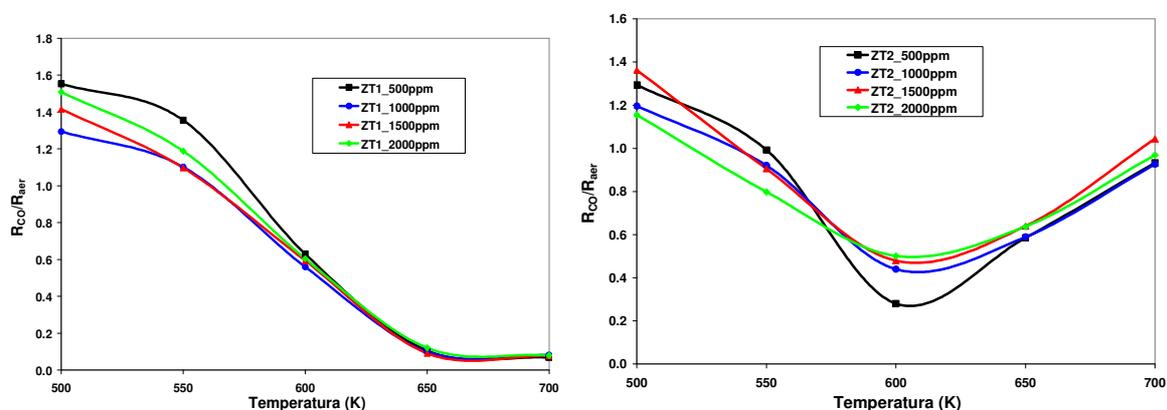
Fig. 9 The sensitivity of the films ZT1 (left) and ZT2 (right) at different concentrations of CO in air
