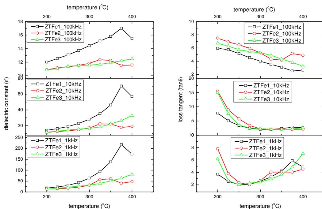
Fig. 12 Variation of dielectric constant (left) and loss tangent (right) of samples ZTFe1, ZTFe2 and ZTFe3 with frequency at different temperatures
