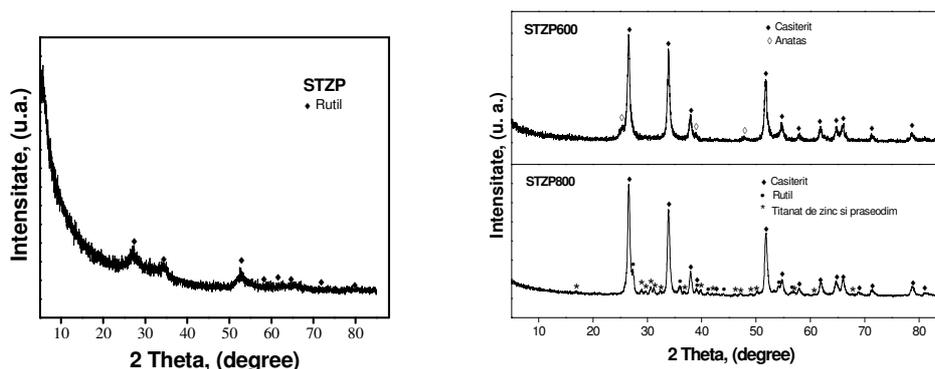
*Fig. 1 X-ray diffraction patterns of films (left) and powders (right) STZP*
