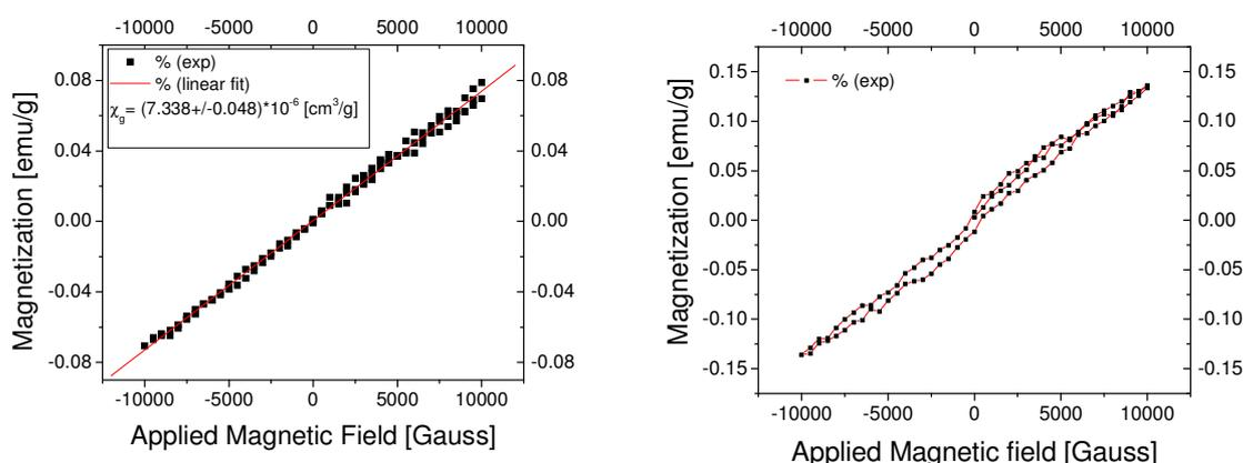
Fig 7. Magnetization of the sample: SZFe1 (left) and SZFe2 (right)
