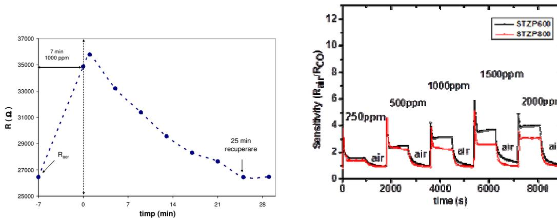
Fig. 3 Recovery time from the different concentrations of CO films (left) and powders (right) STZP
