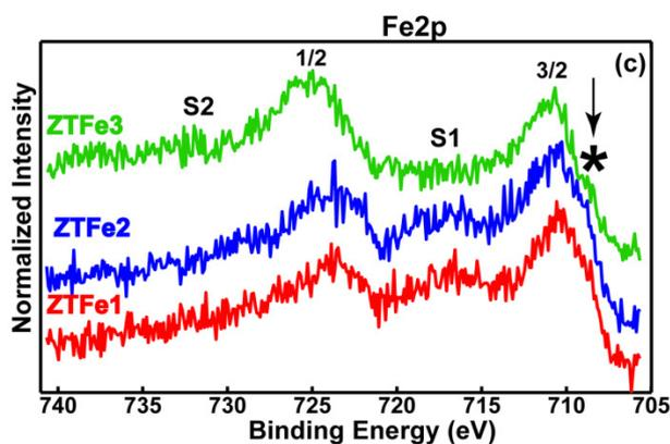
Fig. 10 The superimposed XPS spectra of Fe2p for samples ZTFe1, ZTFe2 and ZTFe3
