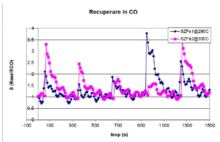
Fig.5 The recovery time of sensors SZFe1 and SZFe2
