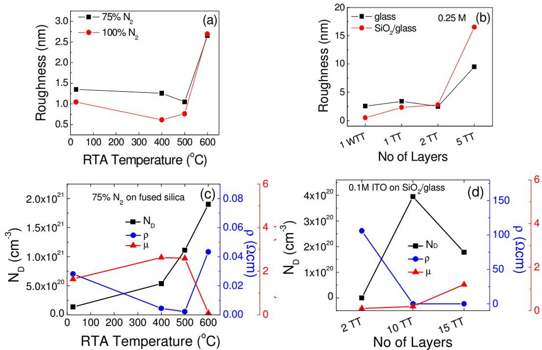
Fig. 13 Roughness (a, b), carrier concentration, resistivity and mobility (c, d) of sputtered (left) and sol-gel films (right)
