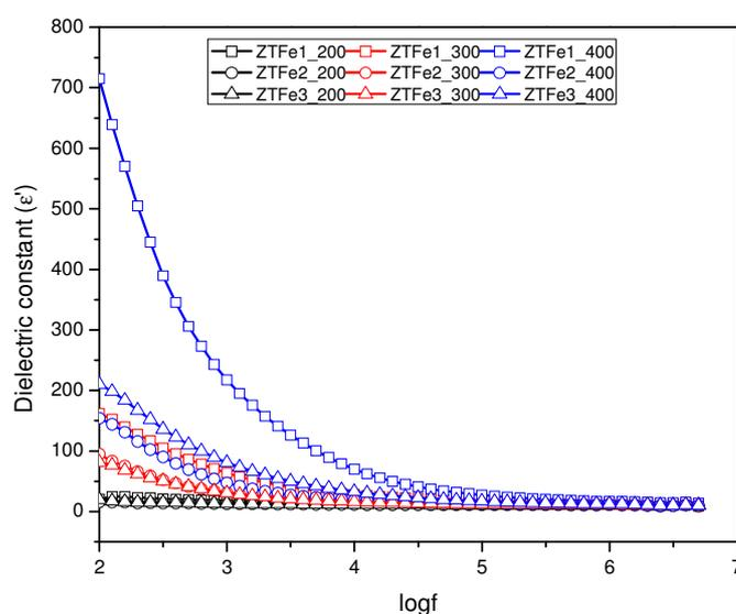
*Fig. 11 The variation of the dielectric constant with frequency for the samples ZTFe, 1 ZTFe2 and ZTFe3 at different temperatures*
