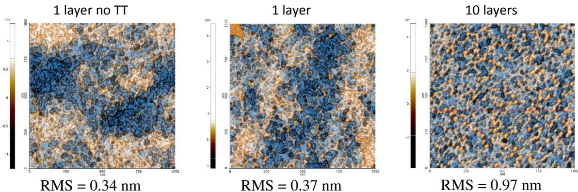
*Fig. 14 AFM 2D images (in high contrast format) of Nb-doped TiO<sub>2</sub> films*
