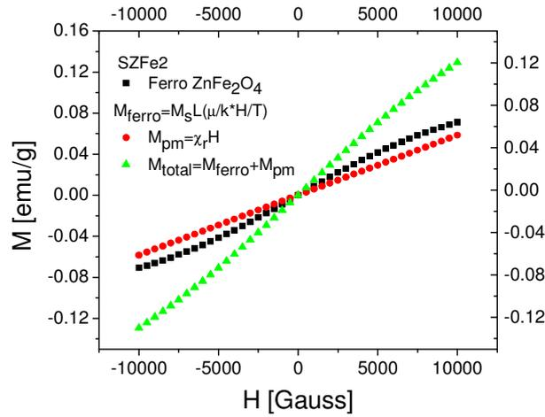
Fig. 8. Magnetization of the SZFe2 sample: ferro, para and total calculated contributions
