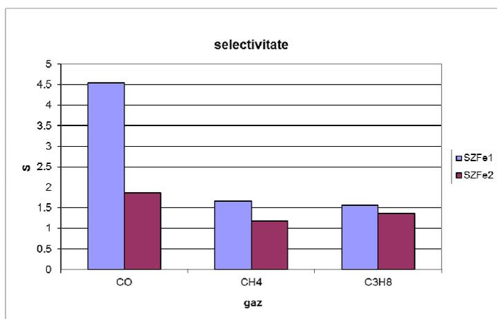
Fig. 6 Selectivity of sensors SZFe1 film and SZFe2 film
