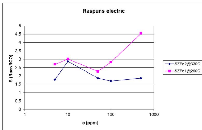
Fig. 4 Sensitivity to CO of sensors SZFe1 and SZFe2
